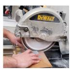
Make sure the wet saw has abundant water flow and cut slowly at 30 seconds or more per inch. Use a new piece of cardboard for cutting each tile. Keep saw table clean.
