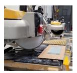
With tile face up, place a piece of cardboard between the glass tile backing and the wet-saw table. The cardboard keeps the glass from getting scratched.
