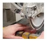
This will remove sediment from the blade without knocking the diamonds off. Cutting a small piece of the stone is all that's needed.
